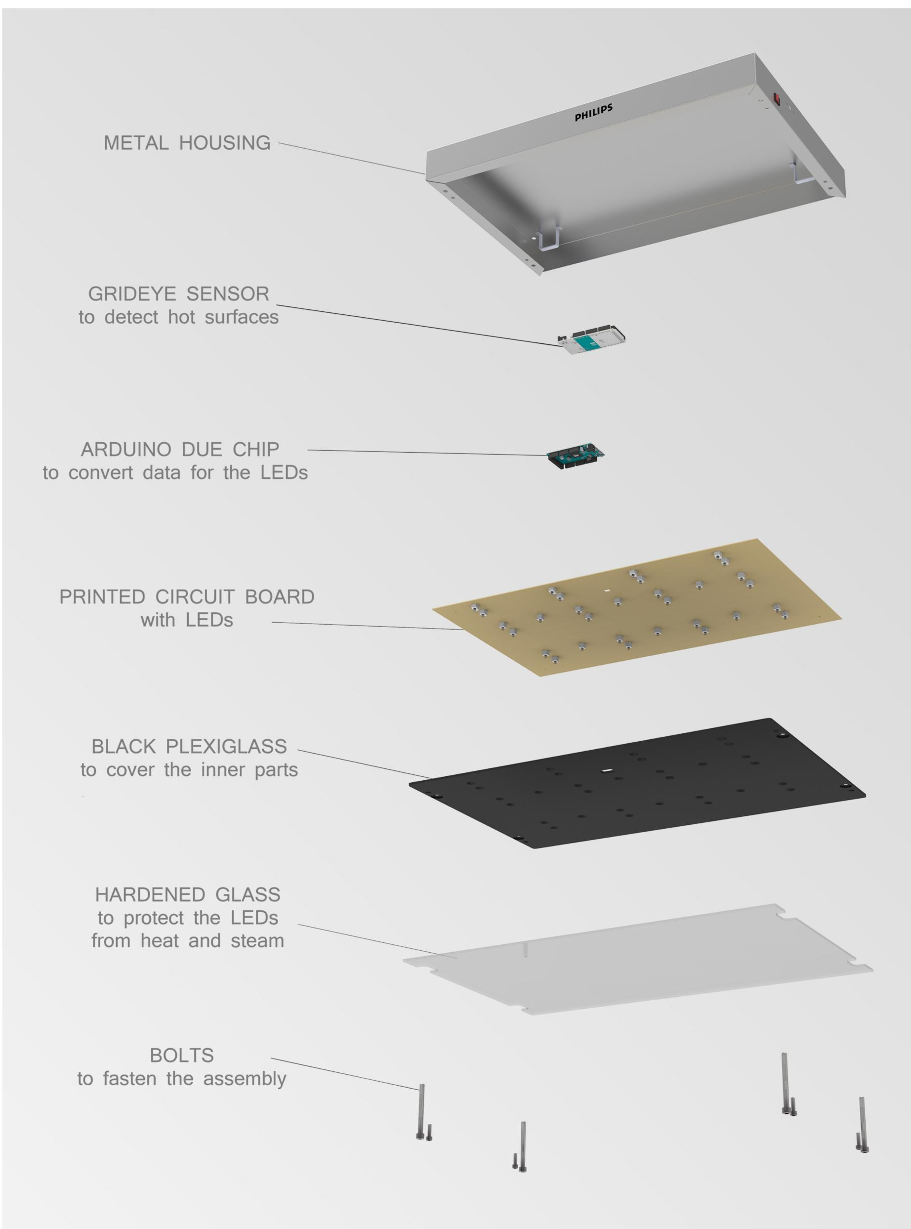
The HOTplate heat detection system consists of several layers.
