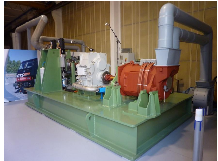
Full-scale test stand for the condition based monitoring of the traction equipment
